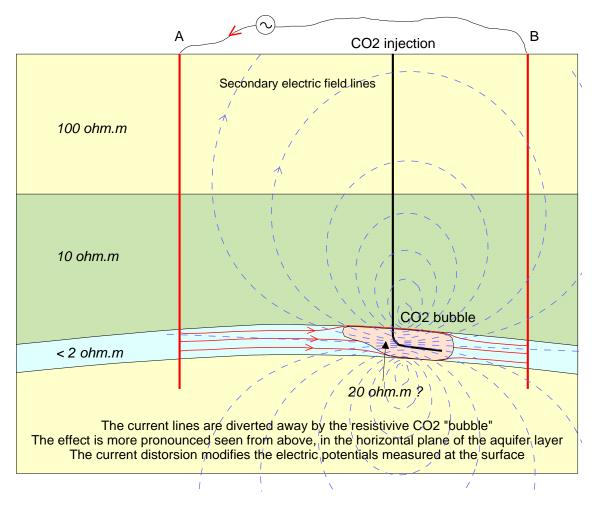
Figure 3 Concept of LEMAM electromagnetic monitoring techniques (BRGM)
