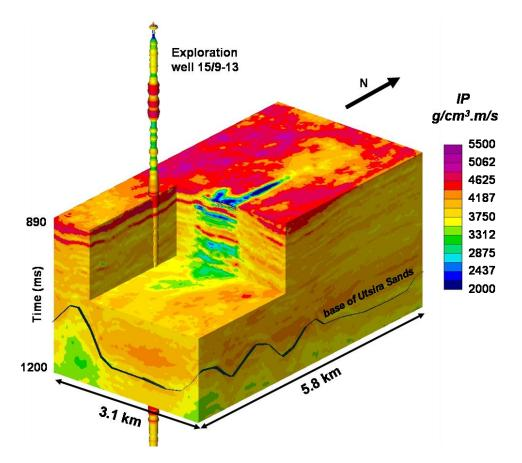
Figure 7 Cut-away view of the 3D P-wave impedance data cube computed by pre-stack stratigraphic inversion of the 2006 vintage. The figure also shows the exploration well used for the calibration step and the intersection between the base of the Utsira Sand formation with the boundaries of the cube. The CO<sub>2</sub> plume is identified by low impedance values displayed in dark blue, blue and green colours (IFPEN).
