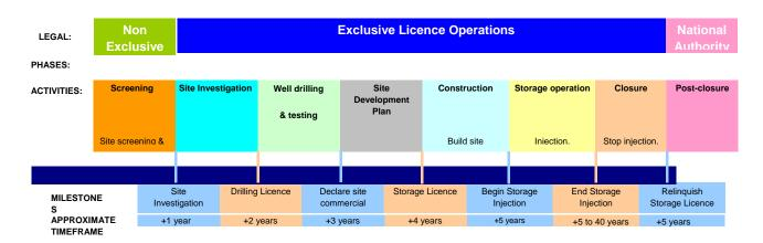
Figure 8 Phases in the realization of a CO<sub>2</sub> storage operation
